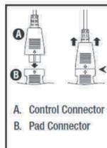
**▲ NOTE:** The Control Connector must be connected to the Pad Connector before plugging the unit into an electrical outlet.
